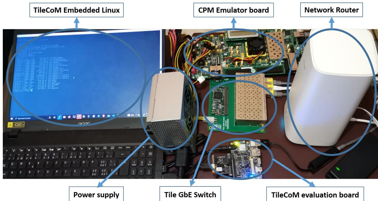
**Figure 5.** *Server and client communication test-bench.*
