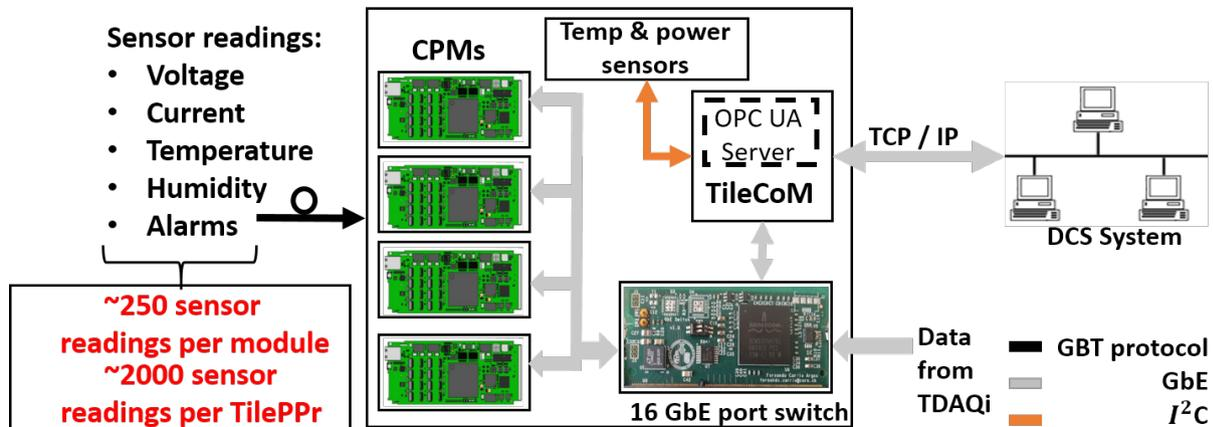
Figure 3. The ATLAS Tile Calorimeter TilePPr-DCS communication system.
