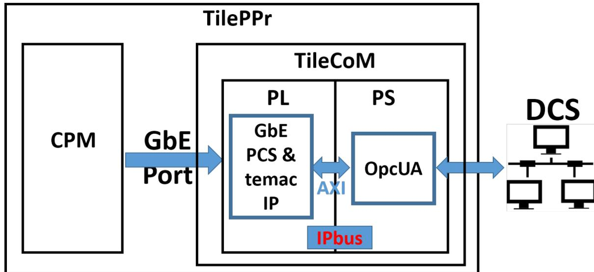
**Figure 4.** The second OpcUA server block diagram for the TilePPr-DCS system.
